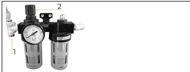
Connect the compressed air supply to the pneumatic unit (1) and set the working pressure with the rotary controller (2) according to the technical data.
